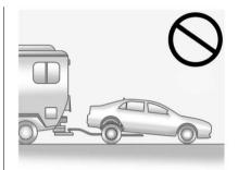
Notice: Towing an all-wheel-drive vehicle with all four wheels on the ground, or even with only two of its wheels on the ground, will damage drivetrain components. Do not tow an all-wheel-drive vehicle with any of its wheels on the ground.
